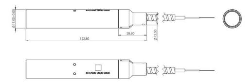
Collimator with isolator. 4mm diameter beam M2<1.2</li>
